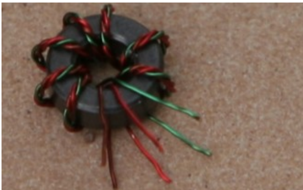
Figure 20. T4/T5 details. FT37-43 core with 8 turns. Sort like colored wires across from each other.
