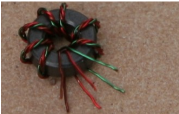
Figure 31. T2 details. FT37-43 core with 8 turns. Sort like colored wires across from each other.
