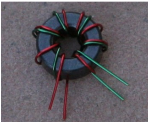
Figure 34. Winding details of T1. 8T red with 6T of green wound over the top of the red windings
