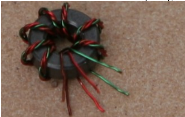
Figure 10. T6 details. FT37-43 core with 8 turns. Sort like colored wires across from each other.
